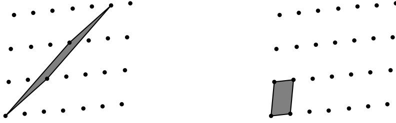
Fig. 1. A lattice and two of its bases represented by the parallelogram they span. The first basis is skew, the second one is minimal (reduced).
