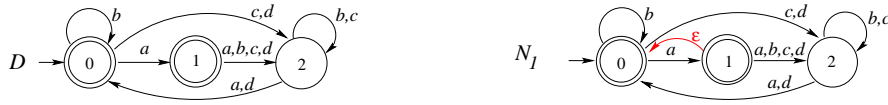
Fig. 1. DFA D for a language L and NFA N_1 for the language L^+ .
