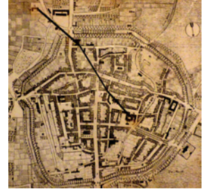
The first electromagnetic telegraph in 1833: a three-kilometer-long wire from Weber's physics lab to Gauss's observatory. ©
