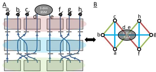
Figure 4. **A:** Two experiments which each create a 3-dimensional 4-photon entangled GHZ state can be combined with a 3-dimensional Bell-State measurement. **B:** In the corresponding graph, the vertices  $d$  and  $e$  are merged. Merging the two graphs can be understood as a generalized multi-photon high-dimensional entanglement swapping.
