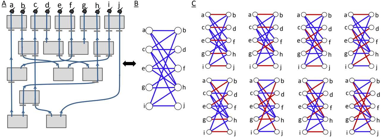
Figure 8. **A:** An optical setup which corresponds to a bipartite graph. It has ten paths and 15 crystals. **B:** The corresponding bipartite graph. The question how many terms the resulting quantum state will have is asking how many perfect matchings there are in the bipartite graph. **C:** In this example, there are eight perfect matchings, which are represented with red coloured edges.
