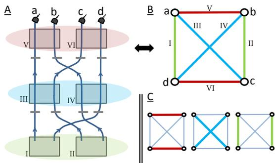
Figure 2. **A:** An optical setup which can create a 3-dimensional 4-photon GHZ-state with the method of Path Identity. It consists of three layers of crystals, in between there are variable mode- and phase-shifters (depicted in grey). **B:** The corresponding graph with four vertices (one for each path), six edges (one for each crystal). Every layer of crystals leads to a four-fold coincidence count. **C:** That corresponds to a *perfect matching* or *1-factor* in the graph.
