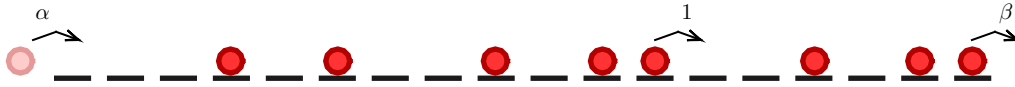
Figure 1. The TASEP. Particles enter at rate \alpha , hop right at rate 1, and exit at rate \beta . The exclusion property means that particles can not overtake each other.
