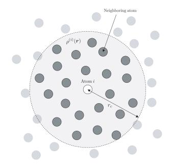
FIG. 1. Schematic illustration of the neighboring atomic density around atom i in a structure composed of a single element.
