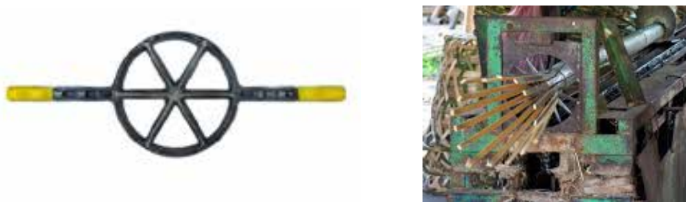
Figure 8 Knives and machines for splitting bamboo [16]. a. hand-operated tool moved to split a fixed culm. b. Bamboo splitting machine with fixed knife and moving culm.
