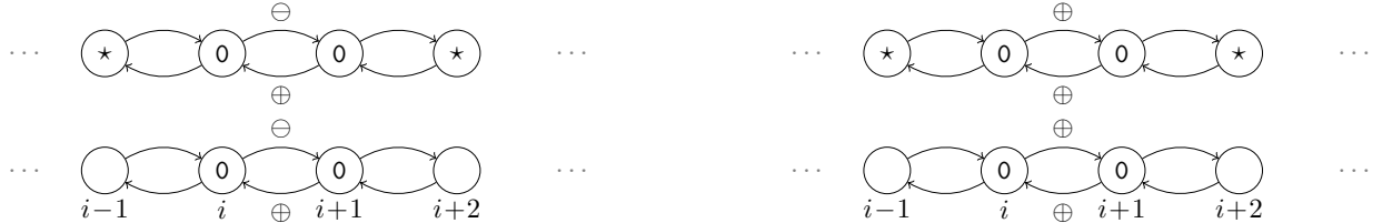
Figure 13: on the left, starting from a configuration (\star, 0, 0, \star) the \Delta update updates before the cell i which becomes 0, after the rule is applied on the cell i + 1 ; on the right, the two cells are updated at the same time or after. In fact, we know that r_{140}(\star, 0, 0) = 0 and r_{140}(0, 0, \star) = 0 .
