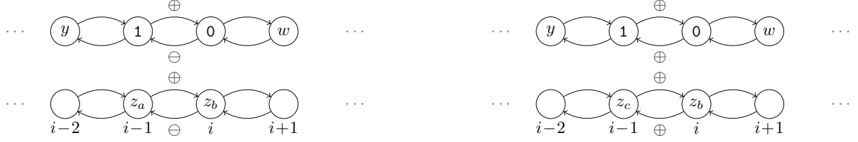
Figure 5: on the left, starting from a configuration (y, 1, 0, w) the schedule \Delta updates before the cell i to z_b = r_{44}(1, 0, w) , after the rule is applied on the cell i - 1 to obtain z_a = r_{44}(y, 1, z_b) ; on the right, the two cells are updated at the same time or after, therefore z_c = r_{44}(y, 1, 0) and z_b = r_{44}(1, 0, w) .
