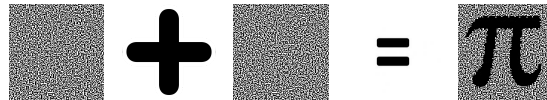
Figure 5: Example of visual cryptography, superposing the images let the symbol \pi appear.
