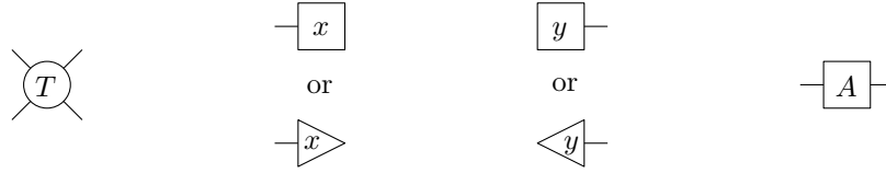
FIGURE 1. In the diagrammatic notation, tensors are represented by boxes. From left to right: a 4-tensor T \in (\mathbb{C}^d)^{\otimes 4} ; a vector x \in \mathbb{C}^d ; a dual vector y \in (\mathbb{C}^d)^* ; a matrix A \in \mathcal{M}_d(\mathbb{C}) .
