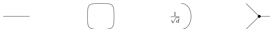
FIGURE 4. From left to right: the identity matrix; loops correspond to the scalar d = \dim V ; a maximally entangled state \Omega = \frac{1}{\sqrt{d}} \sum_{i=1}^d e_i \otimes e_i ; an un-normalized GHZ state \text{GHZ} = \sum_{i=1}^d e_i \otimes e_i \otimes e_i .
