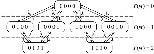
Fig. 2. State space  $\mathcal{W}$  for a minimally connected recovery scheme where  $n = 4$ , showing transition rates and partitioned into subsets  $\mathcal{W}_m$  based on the value of  $F(\mathbf{w})$ .
