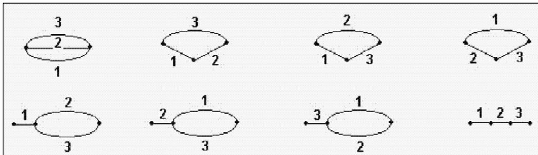
Figure 3: There are 8 labeled series-parallel networks with 3 edges, that is,  $v_3 = 8$ . The “essentially parallel” networks constitute the first row and the “essentially series” networks constitute the second row.
