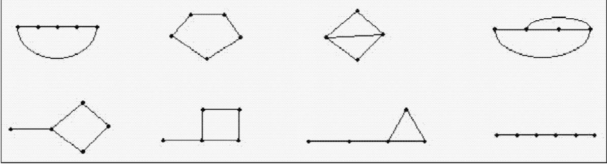
Figure 4: There are 8 unlabeled series-parallel networks with 5 edges that obey the prohibition against multiple parallel edges, that is,  $q_5 = 8$ . The “essentially parallel” networks constitute the first row and the “essentially series” networks constitute the second row.
