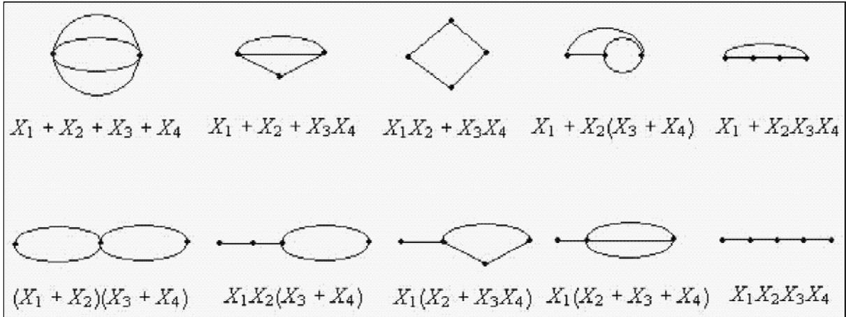
Figure 2: There are 10 unlabeled series-parallel networks with 4 edges, that is,  $u_4 = 10$ . The “essentially parallel” networks constitute the first row and the “essentially series” networks constitute the second row.
