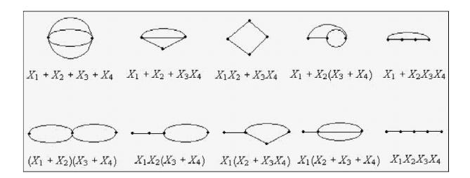
Figure 2: There are 10 unlabeled series-parallel networks with 4 edges, that is,  $u_4 = 10$ . The "essentially parallel" networks constitute the first row and the "essentially series" networks constitute the second row.
